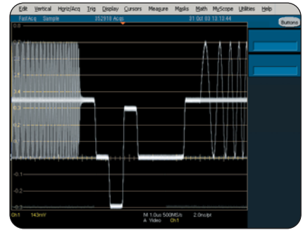
► Video Design. Illustration of triggering on an analog HDTV tri-level sync signal and examining horizontal blanking interval.
