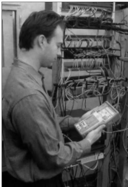
Model 10T1 in use monitoring DS0 channels
