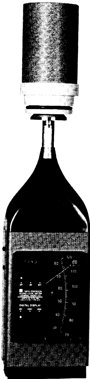
Figure 2-2. Calibration, with the 1567 Sound-Level Calibrator.
