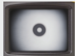
FT300 FiberInspector (250x) shows clear image of multimode fiber end-face ferrule
