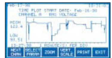
Time Plots Displays a graph of the selected parameter since recording began. ■ Record up to 30 days with internal memory (expandable) ■ Select from up to 16 different parameters ■ Select individual channels ■ Zoom in for greater detail down to 0.1 s/div
