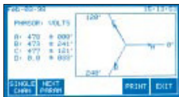
Meter Mode A true three-phase volt-ampere-power-harmonic meter lets you view values updated every second. ■ V, A, W, VA, VAR, power factor, frequency, voltage unbalance, voltage and current THD, current crest factor, K factor, demand, energy and individual harmonics ■ voltage and current phasor diagrams
