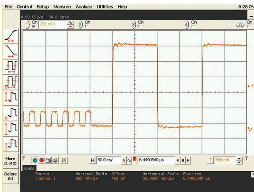
Figure 18. Zoom into the bit level of the D-PHY stimulus signal switching between HS and LP mode
