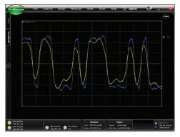
High-fidelity waveform characterization (Yellow: raw trace, Blue: de-embedded waveform)
